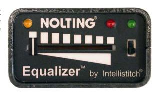
The slider in the middle is used to set the stitch length, when the switch is up, or the constant speed, when the switch is down.
